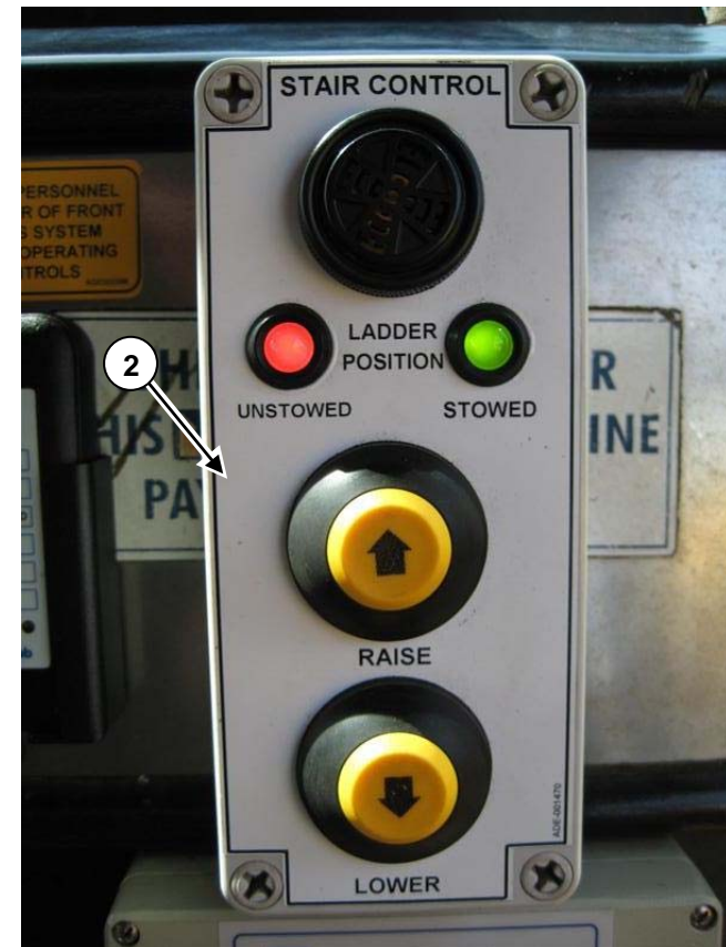
(2) Stair controller on the cab dash
