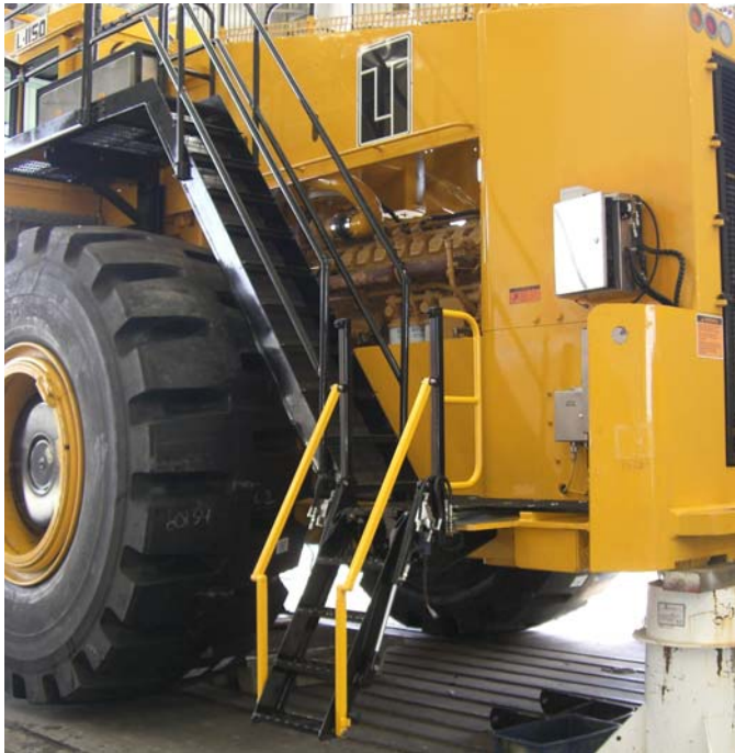
Access system installed on the machine
